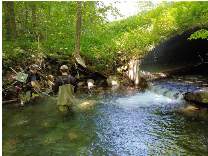
Caption: Electro-fishing on Monday in tributary to Lincoln Brook to count trout below culvert that is currently a barrier to their movement upstream.
